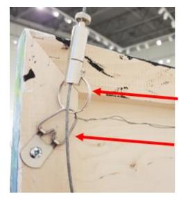
Split rings not smaller than ¾" to easily attach to the wire grips
